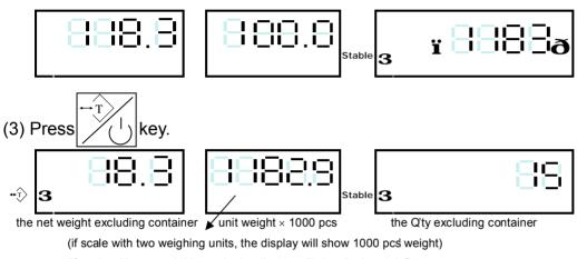
(if scale with one weighing unit, the display will show "unit weight")
